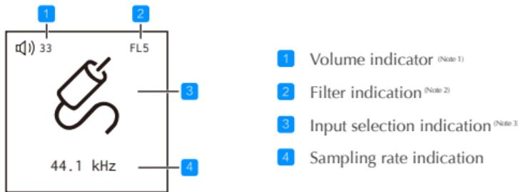
Note 1: When the output volume is set to a fixed volume mode display: Fixed
